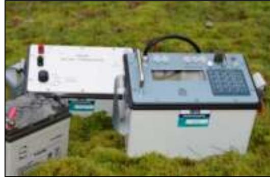
**Fig. 2. the IRIS device used measuring resistivity**
